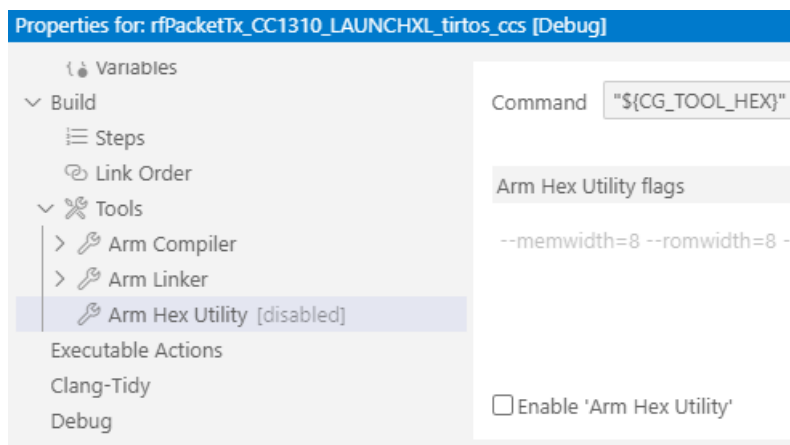
Figure 9: Hex file output is disabled by default. It can be enabled in the build options.
